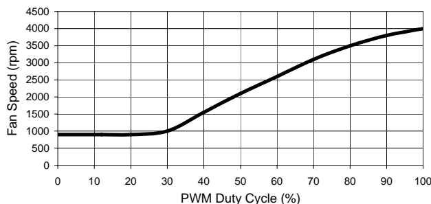
PWM DUTY CYCLE vs. FAN SPEED
